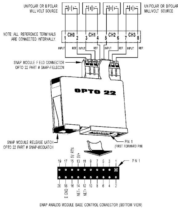
**IMPORTANT:** The mounting rack connector has 24 pins; the module connector has 20 pins. The extra pins on the mounting rack connector prevent misalignment of the module during installation.
